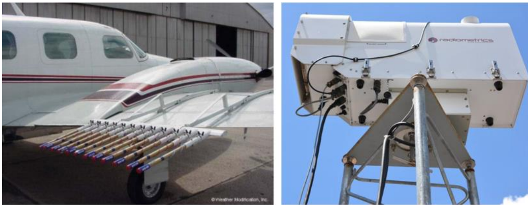
Figure 9. Idaho Power Company cloud seeding aircraft and one of its four radiometers used to target seeding opportunities.
