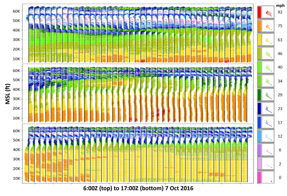
Hurricane Matthew observed by NASA 50 MHz Wind Radar at Kennedy Space Center; eyewall passage 20 km east
