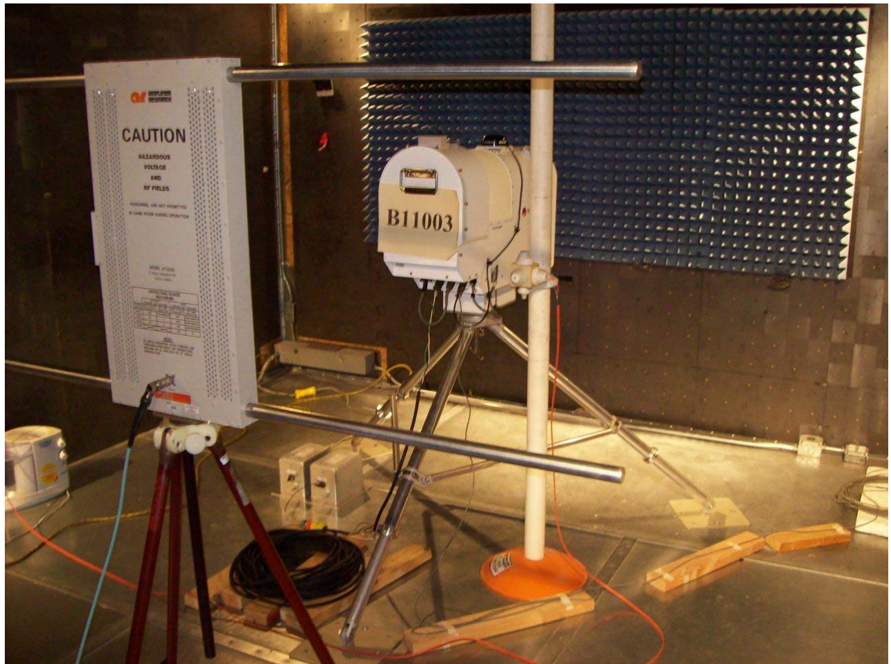
Figure D1. RS103 Test Setup, 2 to 30 MHz.
