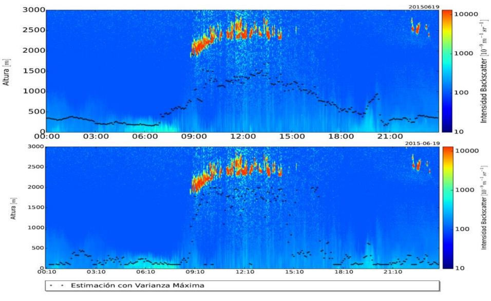
Ceilometer backscatter (color) and boundary layer height (dots) derived from microwave profiler and wind radar (top); and ceilometer only (bottom). The two methods, based on different atmospheric processes, are comparable. *Courtesy of Carlos Hoyos and Laura Herrera* (siata.gov.co/newpage/index.php)
