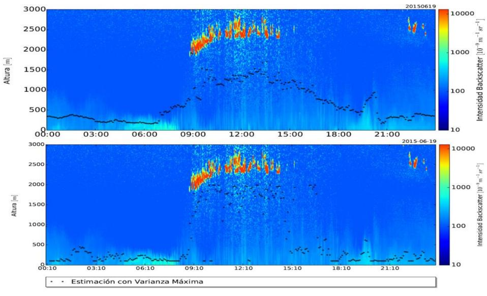
Ceilometer backscatter (color) and boundary layer height (dots) derived from microwave profiler and wind radar (top); and ceilometer only (bottom). The two methods, based on different atmospheric processes, are comparable.
