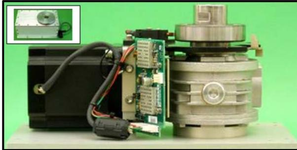
**Figure 10. Azimuth Positioner internal view.**
