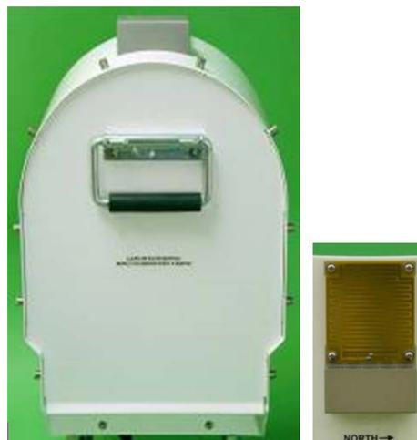
**Figure 6. SuperBlower with access cover installed and Rain Sense Board.**
