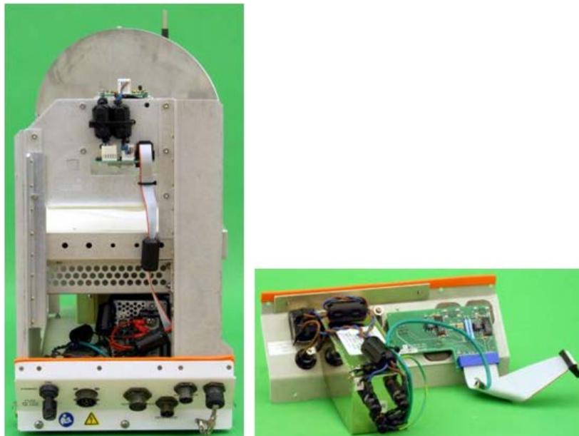
**Figure 8. Field replaceable Power Supply and Front Connector Panel Assembly.**
