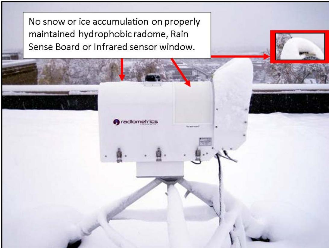
**Figure 2. A Superblower keeps the Radome, Rain Sensor and Infrared Window snow-free.**
