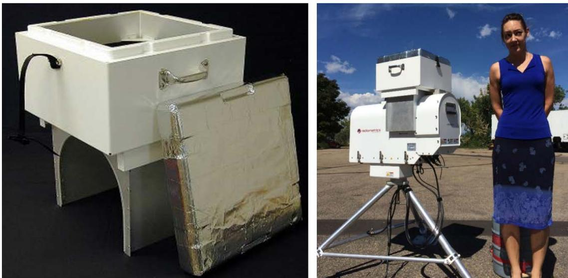
**Figure 9. Patented closed, top-mount Calibration Target ensures optimum accuracy, safety and portability.**
