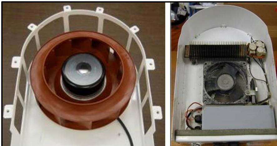
**Figure 3. New SuperBlower with high airflow impeller (left) and old blower with heater (right).**
