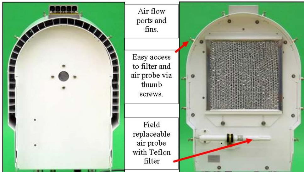
**Figure 4. Superblower back and front (with access cover removed).**
