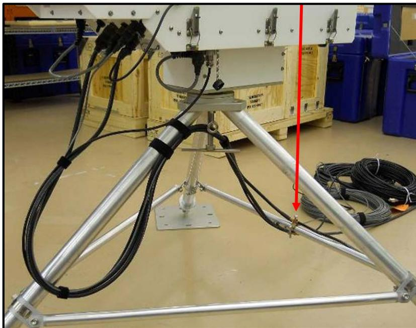
**Figure 11. Tripod for cable routing and earth grounding.**
