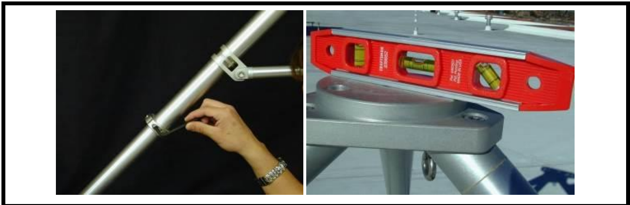
Figure 4: Leveling the TP-2000 Tripod
