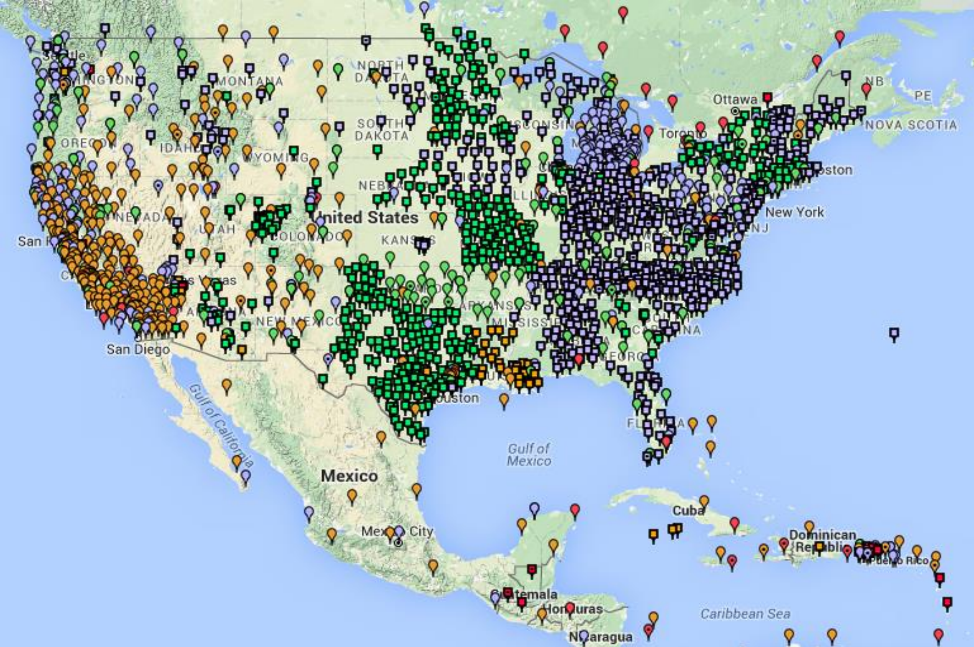
Continuously Operating Reference System (CORS) GNSS Network. The number of network sites and satellites is steadily growing.
