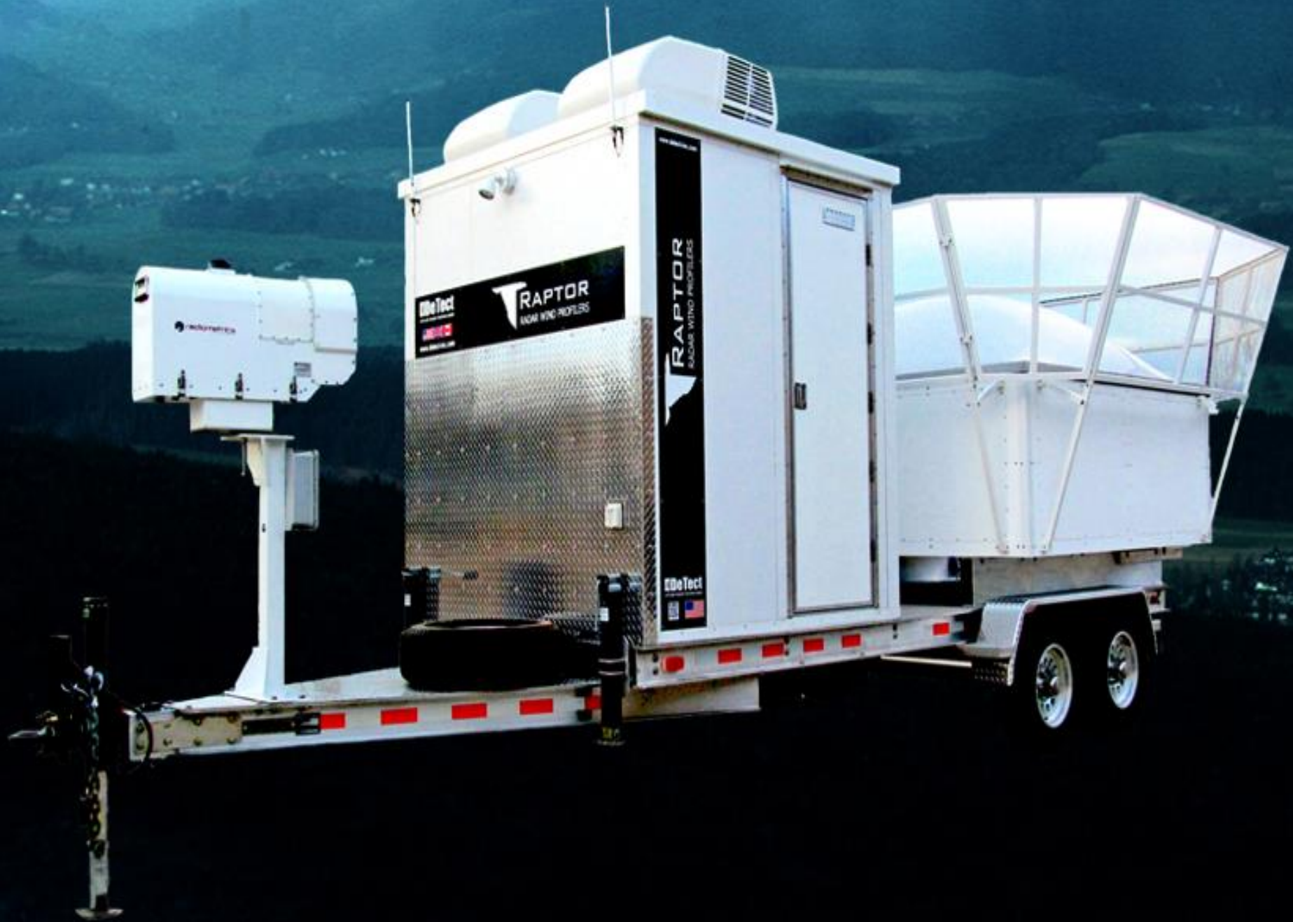
Mobile thermodynamic and wind profiler
