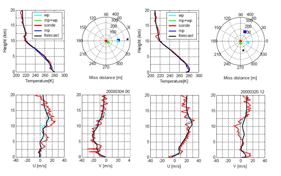
Example radiometer, wind profiler, radiosonde and forecast temperature and wind soundings, and artillery miss distances
