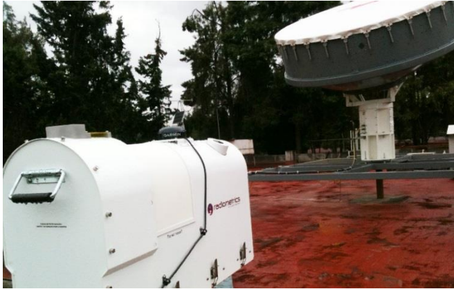
RAPTOR VAD-BL installed alongside a Radiometrics microwave radiometer for a full wind and thermodynamic profiling system (Mexico City).
