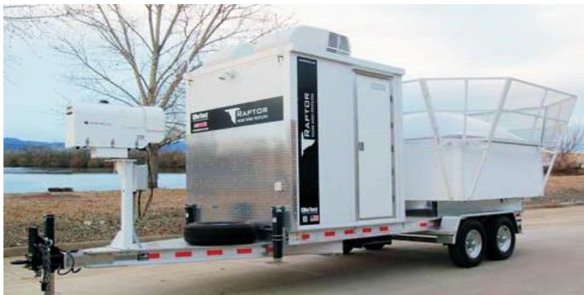
Mobile SkyCast system with RAPTOR® XBS-BL Boundary Layer radar wind profiler
