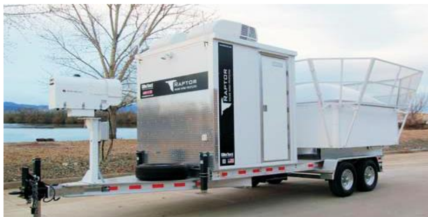
Mobile SkyCast system with an XBS-BL Boundary Layer radar wind profiler
